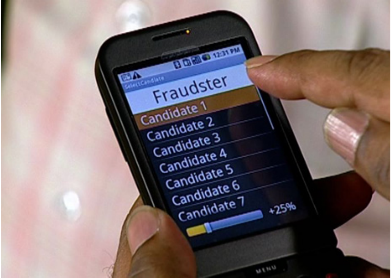
Figure 6: Wireless Signaling — An application running on an Android mobile phone uses Bluetooth to tell our dishonest display which candidate should receive the stolen votes. Attacks using other forms of radio communication are also possible.
