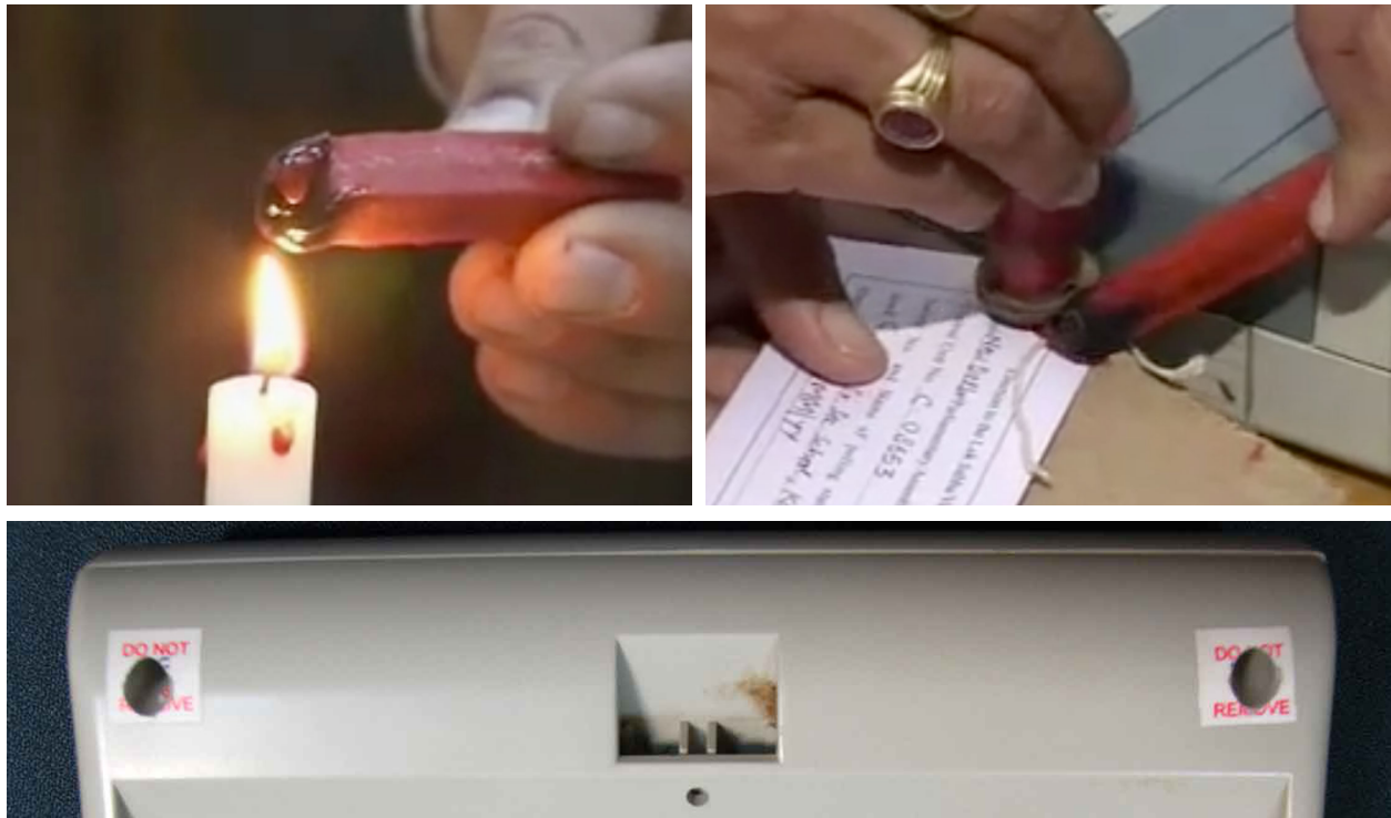
Figure 9: Tamper-Evident Seals — Frames from an official poll worker instruction video [46] ( top ) show how the control unit is sealed with red wax and string. The seals protecting the screw holes on the case ( bottom ) consist of printed paper stickers. Such low-tech seals could be easily faked and provide an extremely weak defense.
