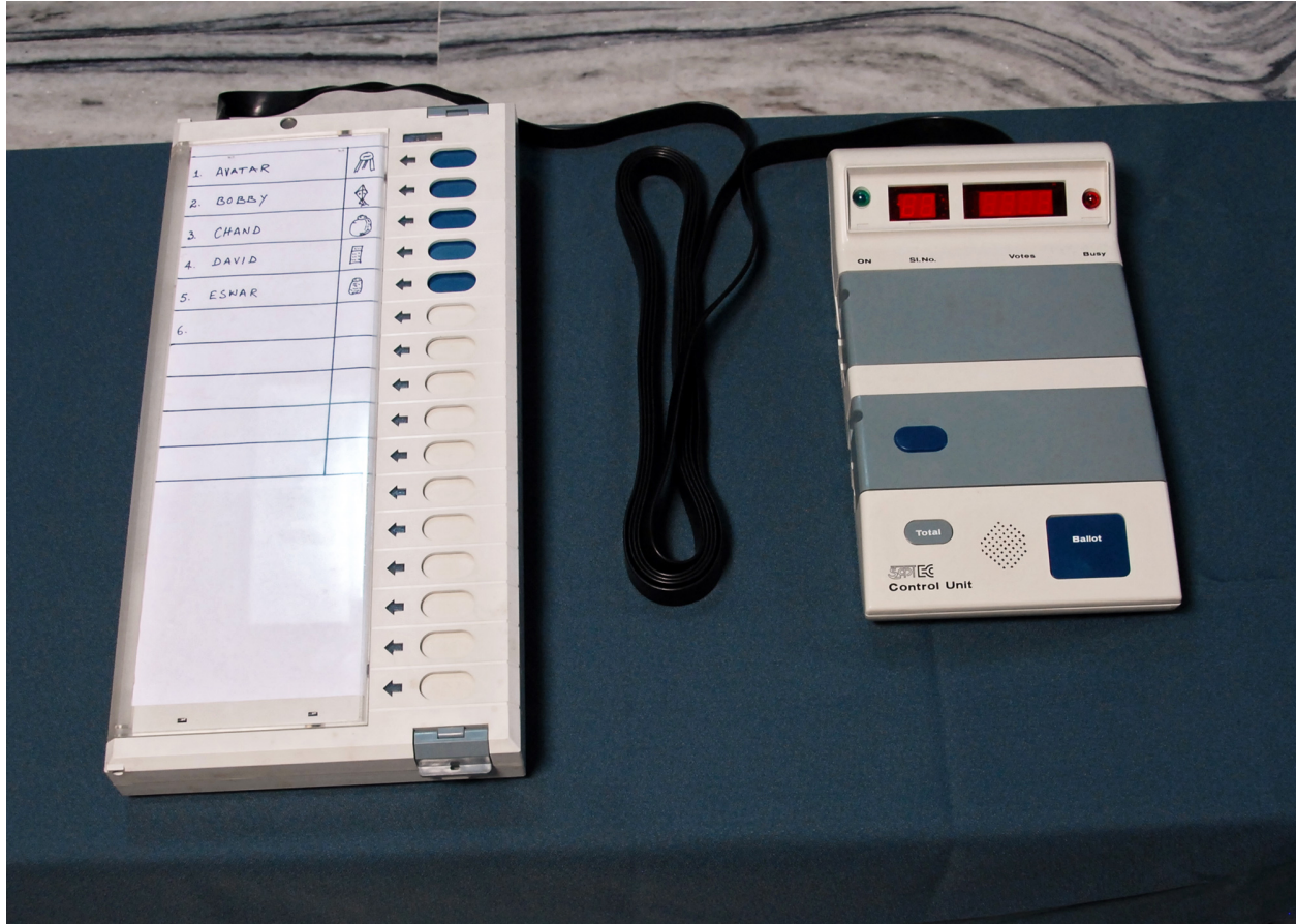
Figure 1: Indian EVMs consist of a BALLOT UNIT used by voters ( left ) and a CONTROL UNIT operated by poll workers ( right ) joined by a 5-meter cable. Inside the election booth, voters simply press the button corresponding to the candidate of their choice. We obtained access to this EVM from an anonymous source.
